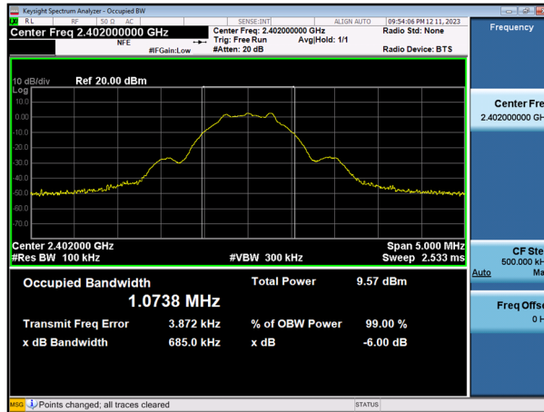
6 dB Bandwidth plot (Mid-CH 19)
