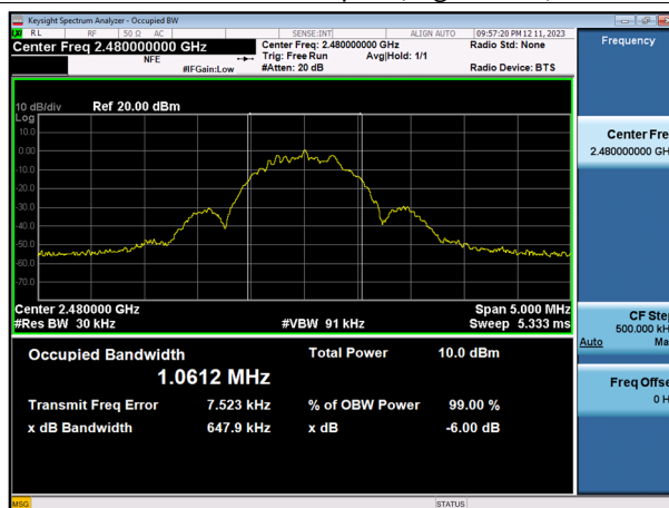
6 dB Bandwidth plot (High-CH 39)
