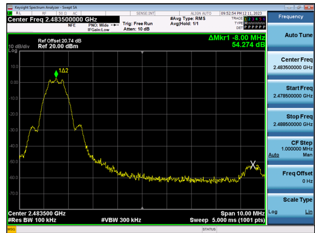
1M Bit/s (255 Byte) High_CH 39
