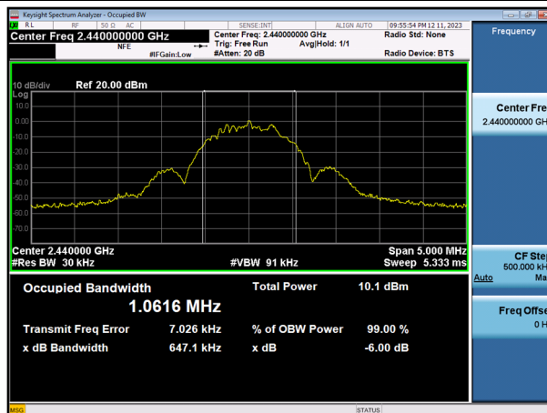
6 dB Bandwidth plot (High-CH 39)
