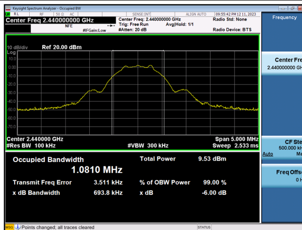
6 dB Bandwidth plot (High-CH 39)
