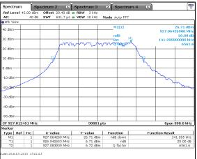
Figure 7.4.4.2-6: 20dB BW High Channel – 4557.3bps
