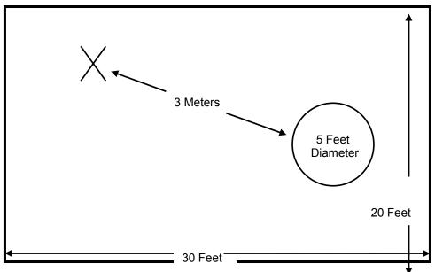
Figure 2.3-1: Semi-Anechoic Chamber Test Site
