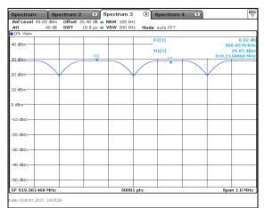
Figure 7.4.1.2-2: Carrier Frequency Separation 4557.3bps
