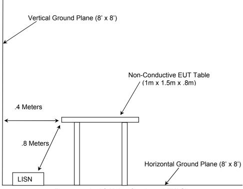
Figure 2.4-1: AC Mains Conducted EMI Site
