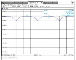
Figure 7.4.1.2-1: Carrier Frequency Separation 2604.2bps
