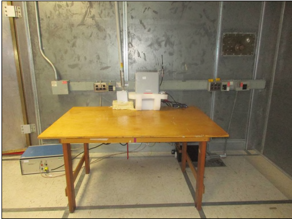
Figure 13: Power Line Conducted Emissions – Front View
