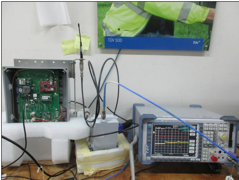
Figure 15: RF Conducted Emissions
