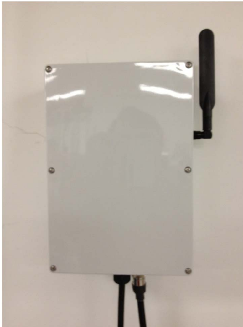
Figure 1: MiHub 1.5 XR with 915 MHz & GPRS.
