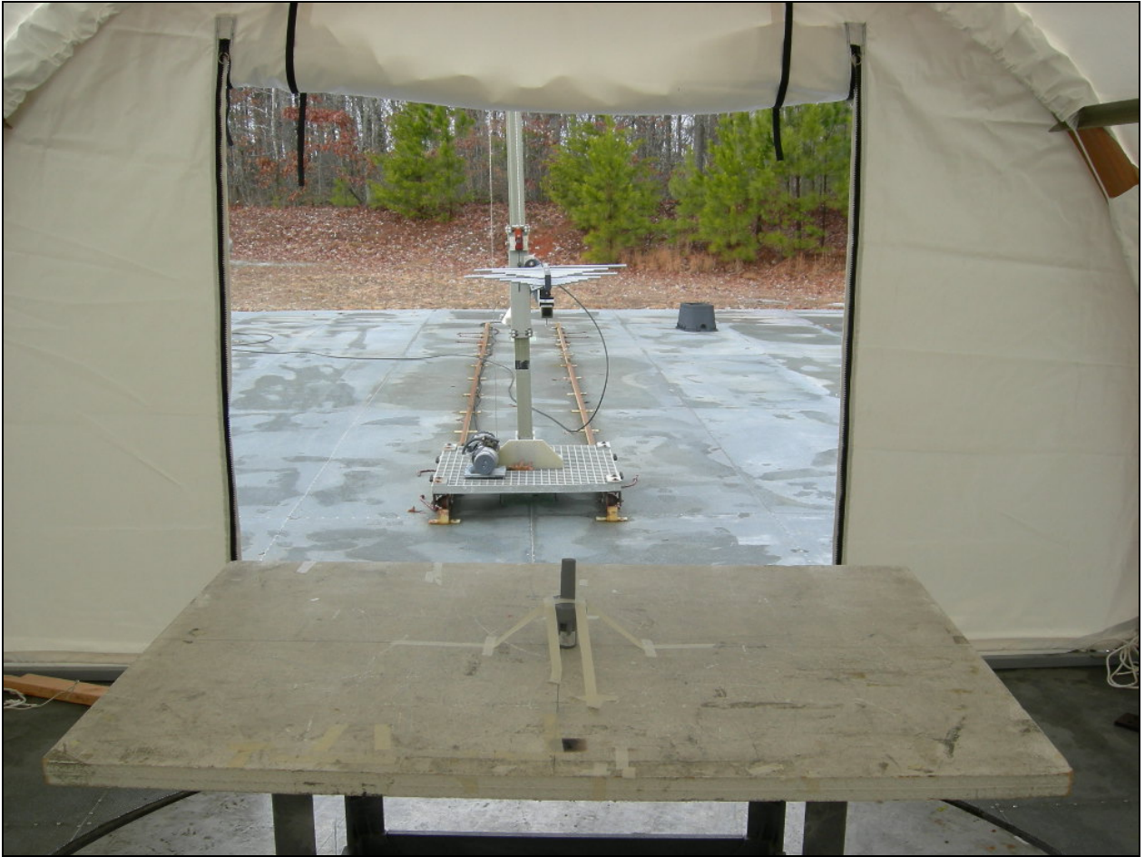
Figure 2: Radiated Emissions - Tabletop Configuration
