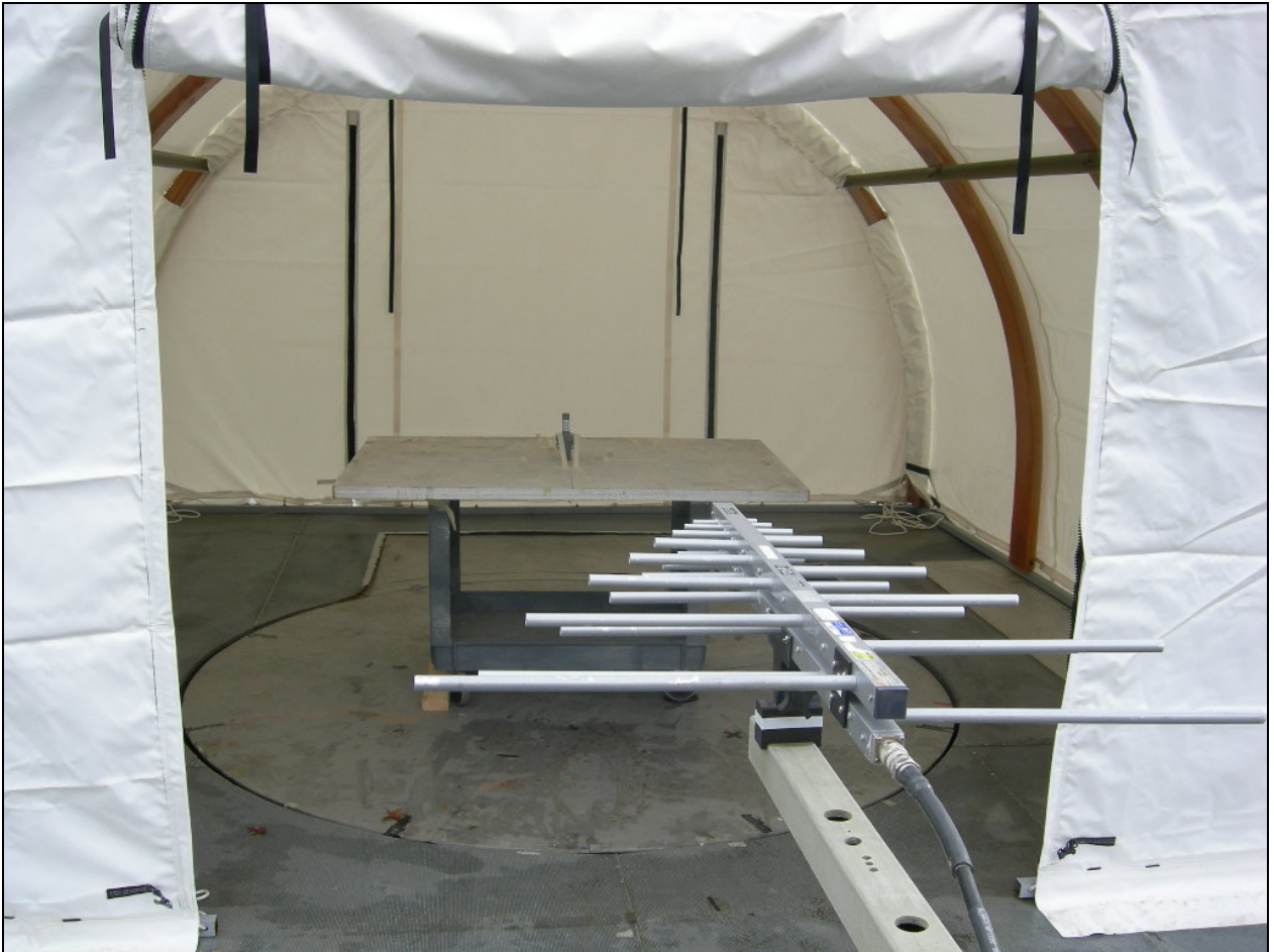
Figure 1: Radiated Emissions - Tabletop Configuration
