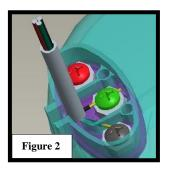
the AMR transmitter will only support the Hersey Translator register and will not work with Hersey's ER, pulse registers. A TRU-Read remote display can be used in conjunction with the Translator register and AMR transmitter for visual remote readings if desired. Refer to TRU-Read installation instructions below to attach both devices. When wiring the TRU-Read to the Translator you must connect the red wire to the red
