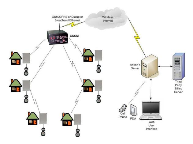
Figure 2.1 Water Meters Connected to ArKion Systems Network
