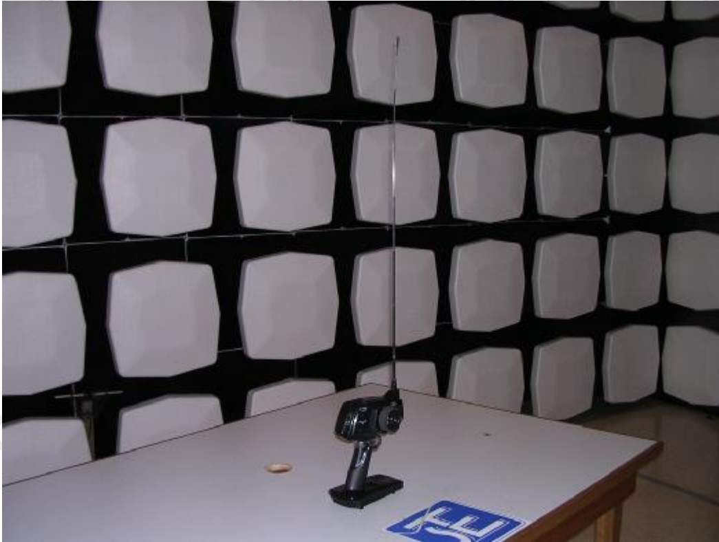
Measurement of Radiated Emission Test Set Up
