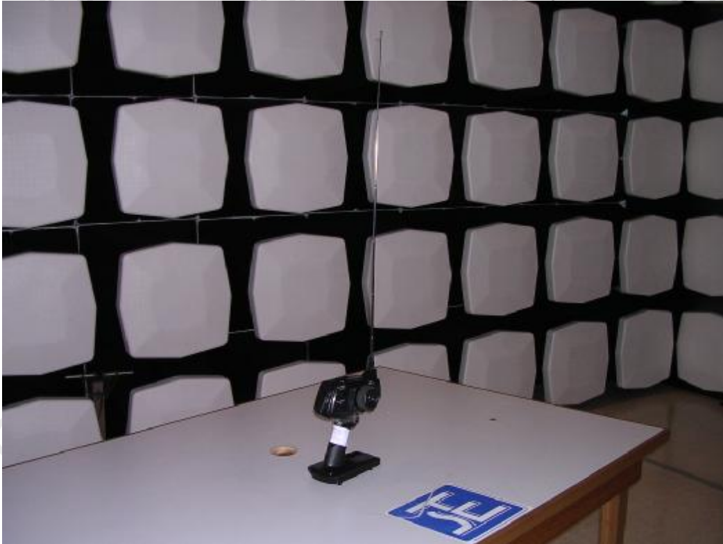
Measurement of Radiated Emission Test Set Up
