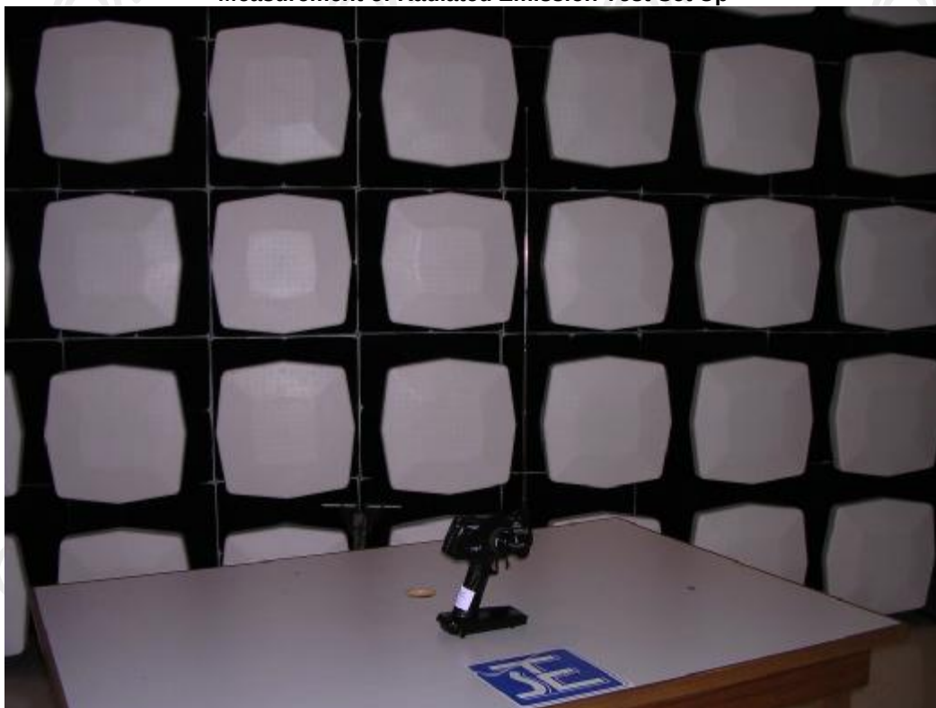
Measurement of Radiated Emission Test Set Up
