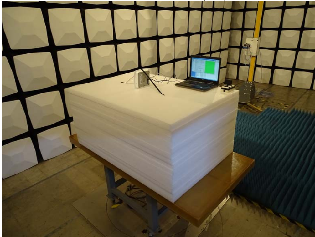
Front View of Radiated Test (Horn)
