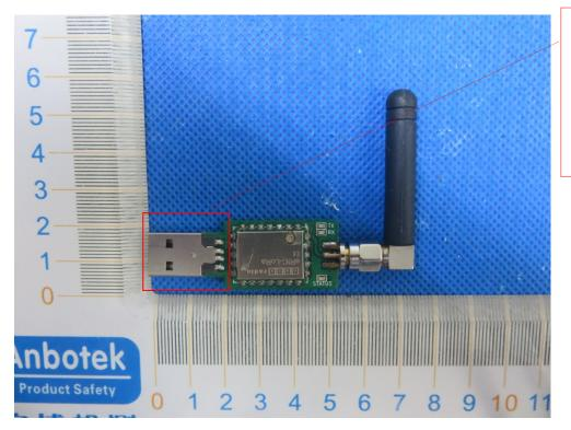
The USB port is for testing purposes only. The EUT itself does not contain a USB port. The final sample shipped is only the module.
