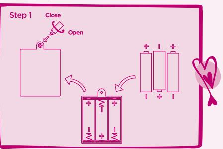
To replace batteries: Unscrew the battery cover and replace 3 x AA (1.5V) size batteries.
