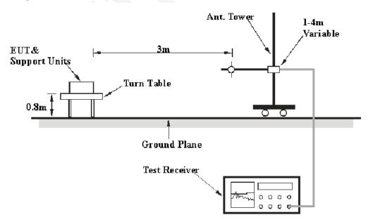
The radiated emission tests were performed in the 3-meter chamber a test site, using the setup accordance with the ANSI C63.4-2009. The specification used was the FCC Part Subpart C limits.
