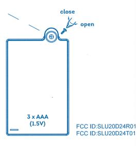
REPLACING REMOTE CONTROL **BATTERIES**
