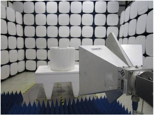
1.2 Radiated Spurious Emissions Test Setup
