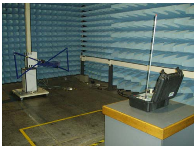
PHOTO N° 2 – SET-UP FOR EMISSION RADIATED TEST
