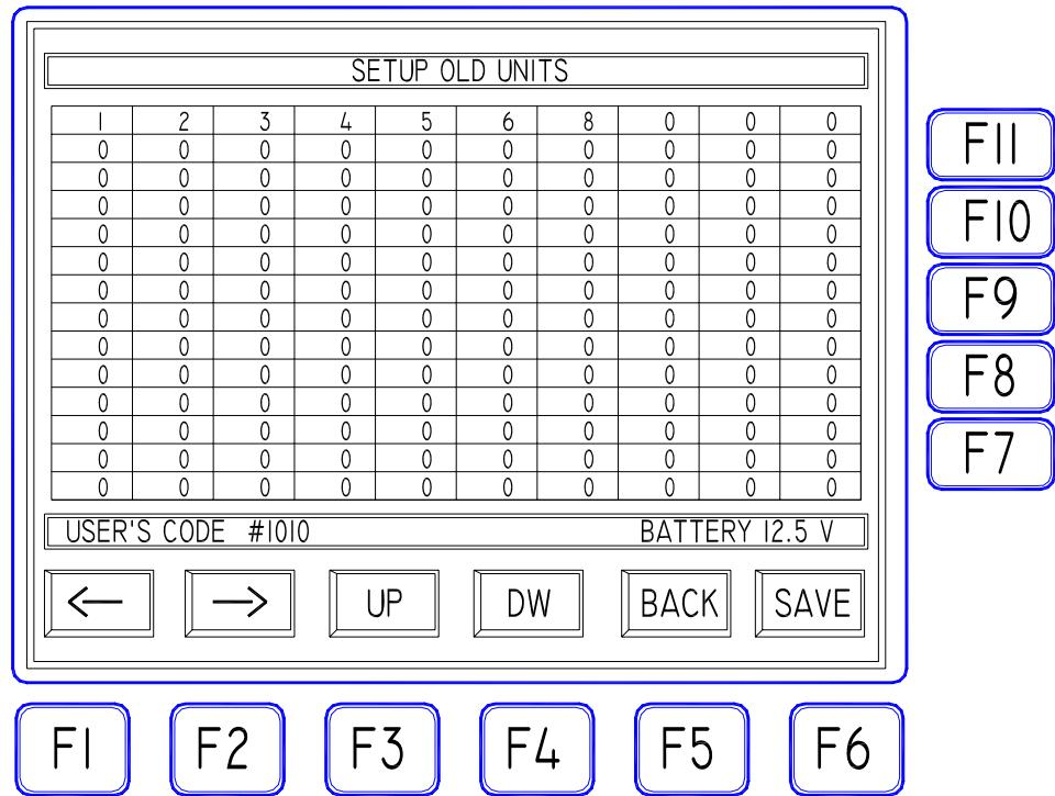
Once the numbers of the "old generation" type Units, will be correctly entered, press the F6 "SAVE" key to confirm and leave the mask using F5 "BACK".
