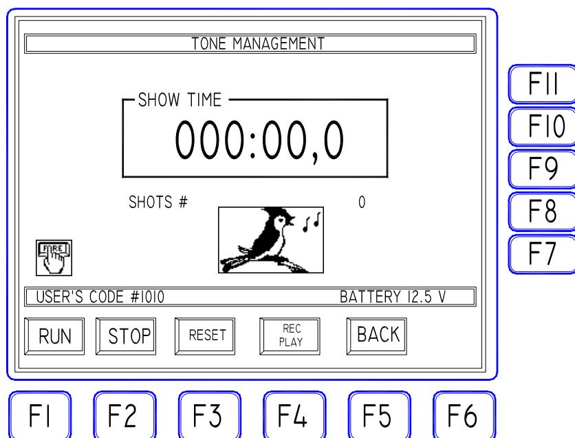
When the "FIRE" key is pressed the first time (start of the show), the time counter (SHOW TIME) starts to advance displaying minutes, seconds and tenths of a second elapsed (up to 999minutes, 59 seconds and 9 tenths). At any time the time counter can be STOPPED ("STOP" F2), RESET TO ZERO ("RESET" F3) and RE-STARTED ("RUN" F1) using the relative function keys. As usual the "BACK" key allows to exit the function and to return to the previous mask.
