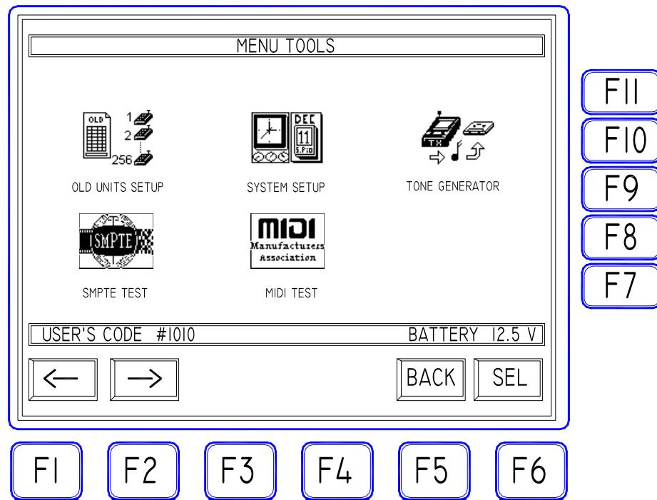
The Icon selection is made by means of the F1 and F2 keys allowing to highlight in sequence the three available icons. with F6 "SEL" key the selected icon will be activated. With F5 "BACK" key the main menu is selected again. Inside this mask all other function keys are disabled.
