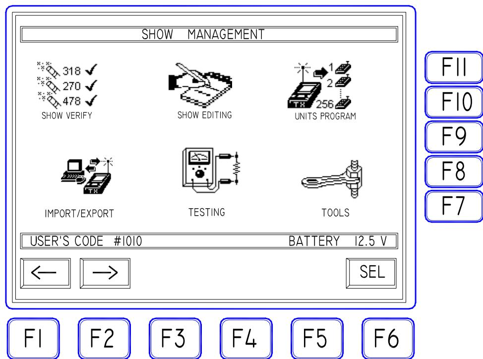
**NOTE** the display back lighting is timed and automatically turns off after 30 seconds. Pressing any key it will turn on again immediately
