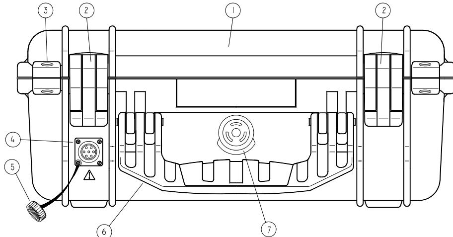
1. IP67 Ultra High Impact Copolymer Polypropylene case. 40.6 x 33 x 17.4 mm
