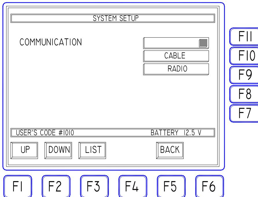
**TRANSMISSION MODE SELECTION:** with "UP" and "DOWN" keys (F1 and F2), select the "COMMUNICATION" bar, press the "LIST" key (F3) to open the pop-down showing the two possible options "RADIO" or "CABLE". Select with "UP" and "DOWN" keys the needed mode and confirm using ENTER. The "BACK" key allows to exit the mask returning to the previous menu.
