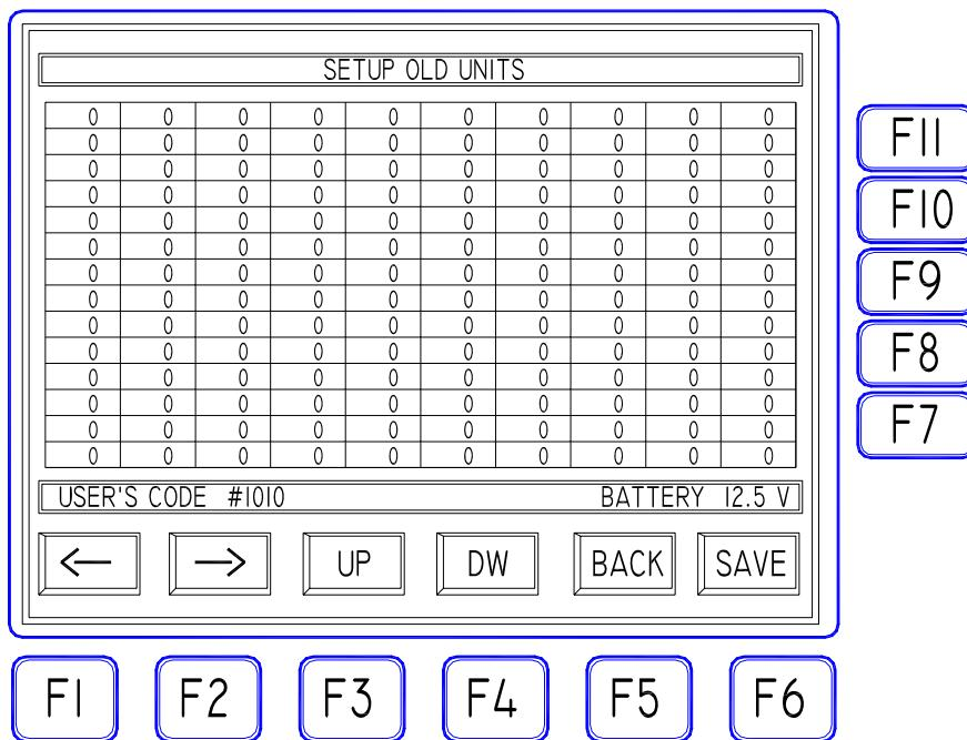
The numbers of the "old generation" type Units, can be inserted IN ANY ORDER and IN ANY CELL among the 140 available. For an obvious readability reason, it is suggested to proceed orderly starting from the **uppermost cell on the left**. One should insert ONLY the numbers of the FIREMASTER II "old generation" Remote Units (RX24), leaving at ZERO all other cell values.
