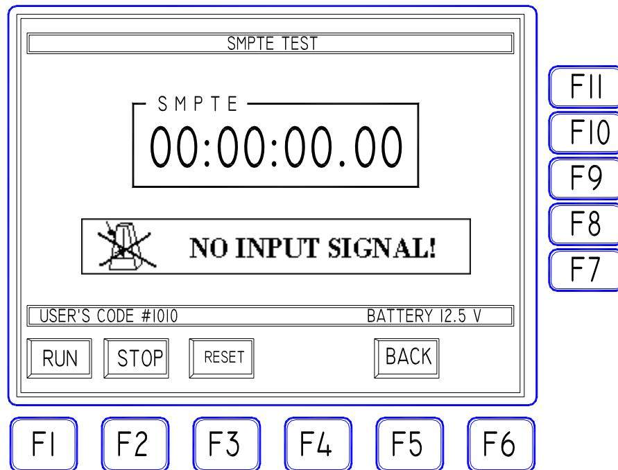
When a valid SMPTE code is applied to the front-panel input and the RUN key pressed, the system will start to decode the incoming signal and the mask will display the "SYNCHRONIZED" message along with the type of SMPTE decoded (24, 25, 30 fps, drop or no-drop). The counter will start immediately to display the actual time code received (hours, minutes, seconds, frames/second):
