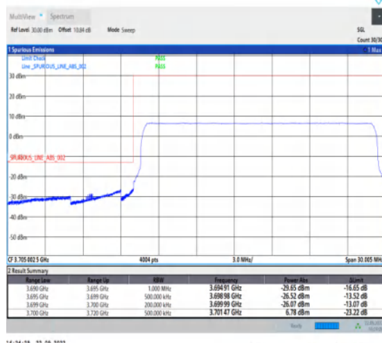
1-N77-3700-3980-PC2-30-20-L-6-CP-QPSK-Outer _Full-51@0-Ant1-1--PASS-see graph
