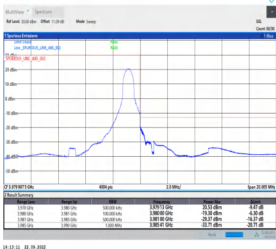
1-N77-3700-3980-PC2-30-10-H-5-CP-QPSK-Edge_1R B_Right-1@23-Ant1-1--PASS-see graph
