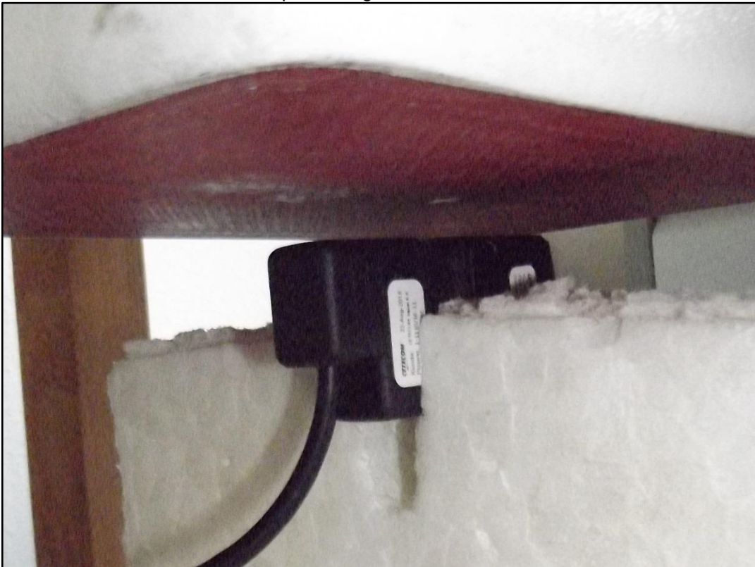
Photo 10: Test position right side with 10 mm distance
