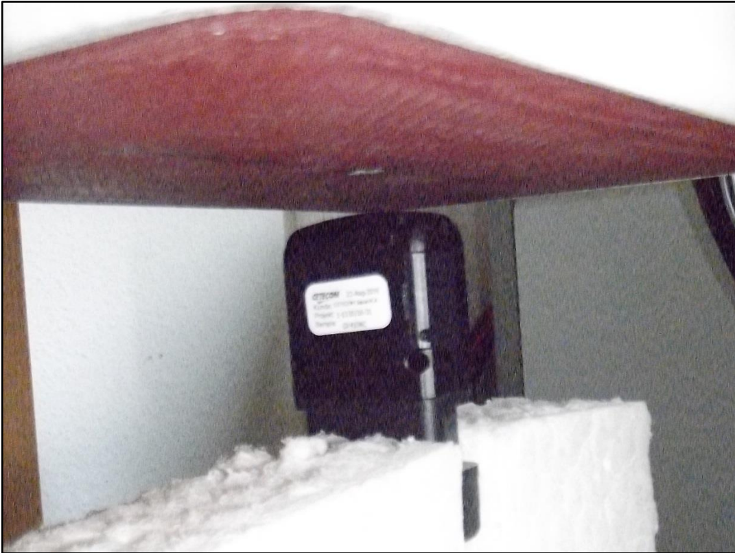
Photo 11: Test position front side with 10 mm distance
