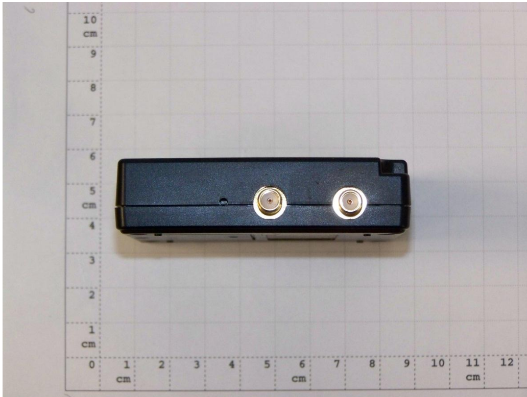
Main EUT A with enclosure (SMA-female connectors side)
