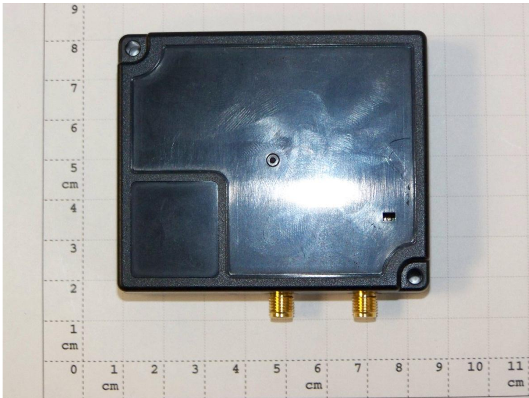
Main EUT A with enclosure (ext. SMA-female connectors, right GPS & at the middle for GSM/UMTS)
