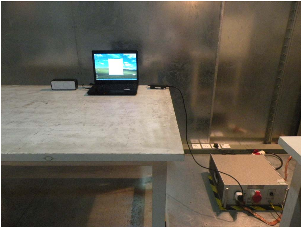
Radiated Emission Test Setup in Chamber
