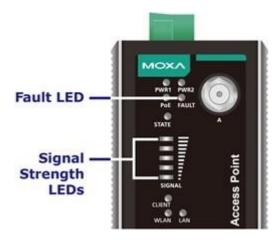
The following table summarizes how to read the device's wireless settings from the LED displays. More information is available in *Chapter 3* in the *Basic Wireless Settings* section.
