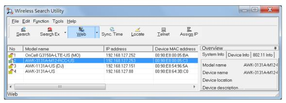
8. Click on the **Telnet** icon if you would like to use telnet to configure the selected device.
