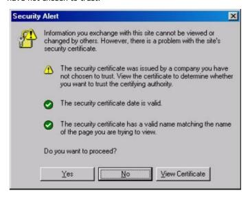
3. Select Yes to accept the certificate issued by Moxa IW and then enter the AWK-3131A-M12-RCC's web browser interface secured via HTTPS/SSL. (You can see the protocol in URL is https.) Then you can use the menu tree on the left side of the window to open the function pages to access each of AWK-3131A-M12-RCC's functions.
