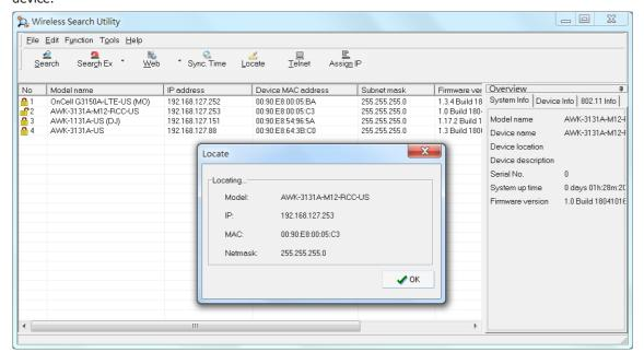
To unlock a specific product without requiring to enter the Username/password each time, go to **Tools** → **Login Options** to manage and unlock multiple products.
