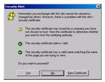
3. Select **Yes** to accept the certificate issued by Moxa IW and then enter the TAP-213's web browser interface secured via HTTPS/SSL. (You can see the protocol in URL is **https**.) Then you can use the menu tree on the left side of the window to open the function pages to access each of TAP-213's functions.
