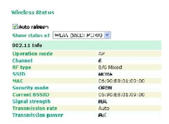
**NOTE** The **802.11 info** that is displayed may be different for different operation modes. For example, "Current BSSID" is not available in Client mode, and "Signal strength" is not available in AP mode.
