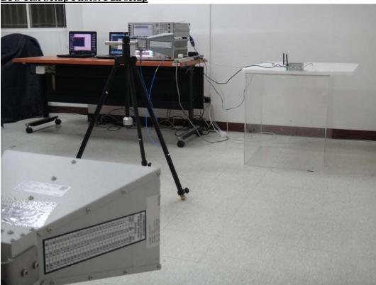
**DFS Test Setup Photo: Client device**
