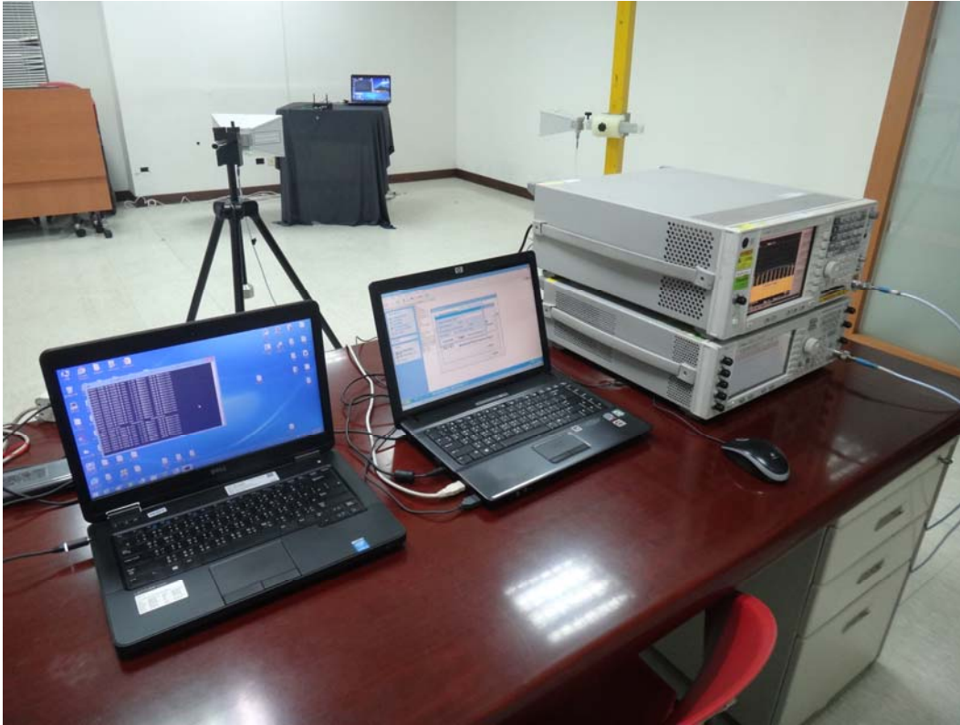
DFS Set-up Photo: Spectrum Analyzer and Radar Generator
