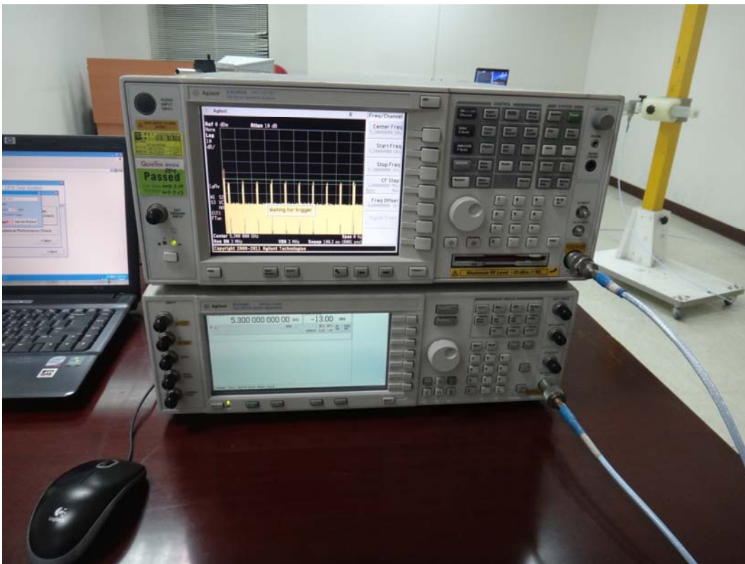
DFS Set-up Photo: Spectrum Analyzer and Radar Generator
