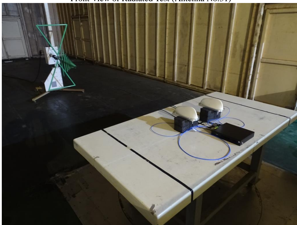
Back View of Radiated Test (Antenna No.31)
