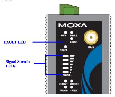
The LEDs for **SIGNAL** are a signal strength indicator and they merely function in **Client** mode.
