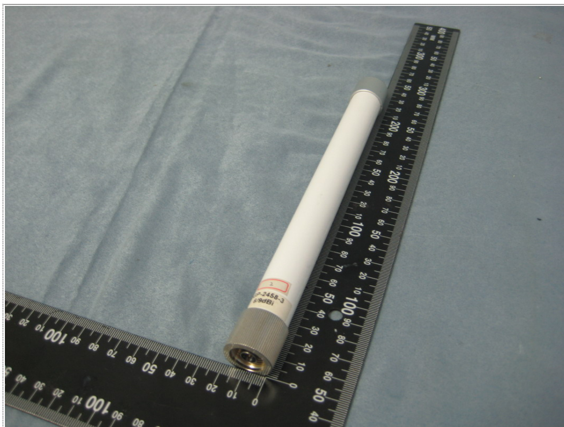
View of Antenna (ANT-WDB-ANM-0609)
