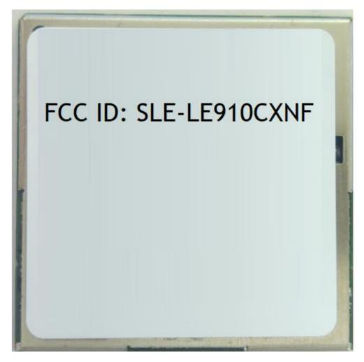
LE910CXNF Label location paste on the shielding
