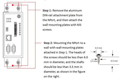
Do not drive the screws in all the way—leave a space of about 2 mm to allow room for sliding the wall-mounting panel between the wall and the screws.
