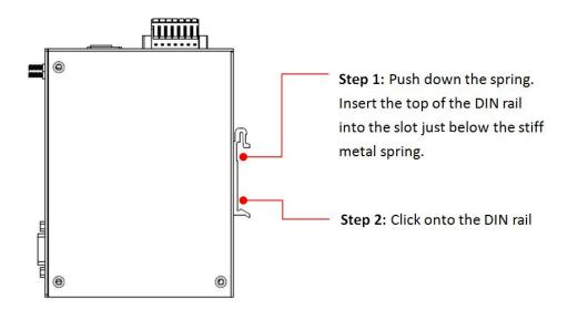
To remove the NPort IAW5x50A-6I/O from the DIN rail, reverse Steps 1 and 2.
