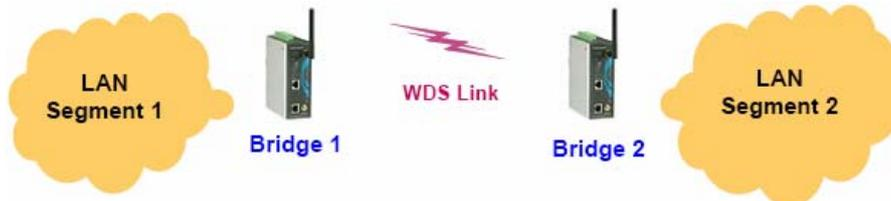
It is a good idea to plan your wireless network by drawing a diagram so that you know how each AWK-3121 is connected to other peer APs or wireless bridges by WDS, and how bridges are connected to other peer bridges by WDS. See the following figure for an example of a network-planning diagram.
