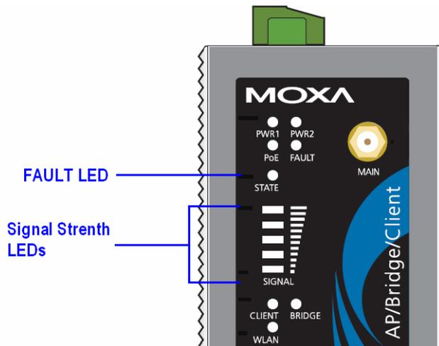
The LEDs for **SIGNAL** are a signal strength indicator and they merely function in **Client** mode.
