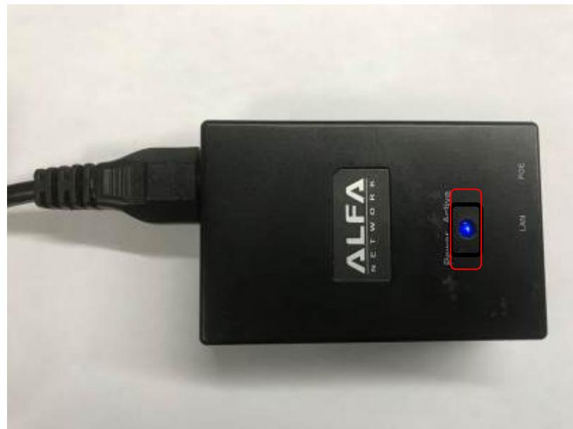
(Step11). The LAN ports Ethernet cable is connect with the “POE port” at the POE adapter.
