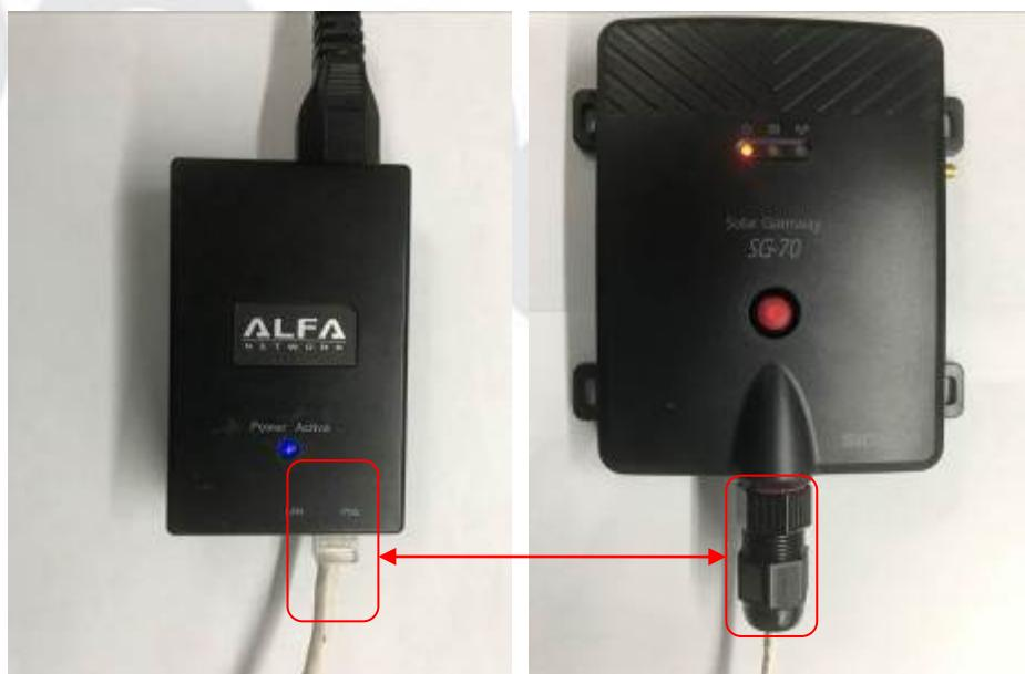
(Step12). The WAN port Ethernet cable is connect with the “LAN port” at the POE adapter and others side connect to the PC or NB.
