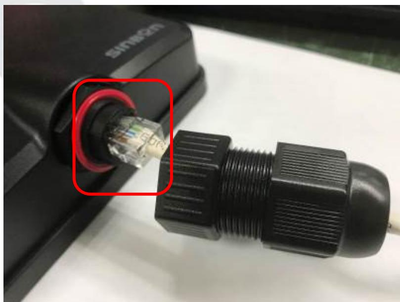
(Step8). First lock the waterproof connector part 3 until to locked, then until locked the part1.
