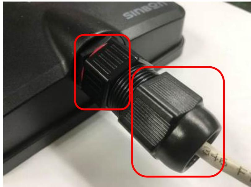
(Step9). The Second LAN cable for WAN port used, after the RJ45 connector front end 12cm, the Ethernet cable around 1 circle on the clamp core.
