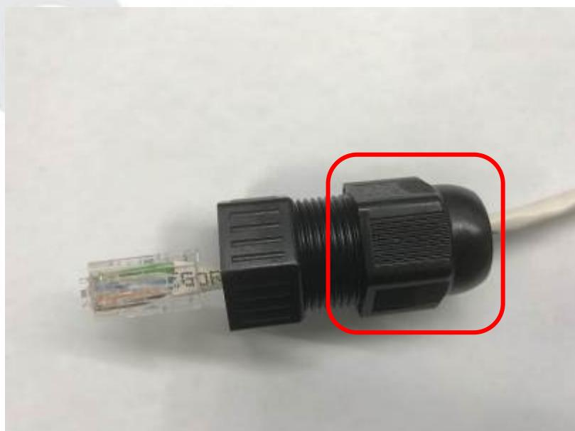
(Step6). The waterproof connector kits part 4 waterproof washer, set on the Ethernet port at the Solar gateway.
