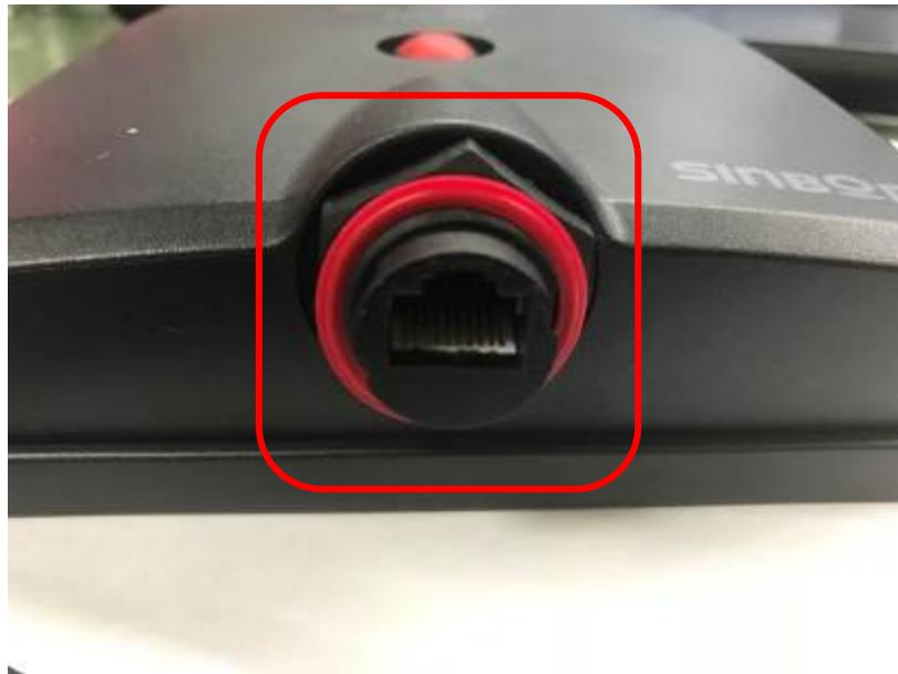
(Step7). Connect the Ethernet cable to the Ethernet port at the Solar gateway.
