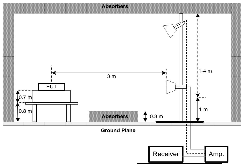
(C) For radiated emissions below 30MHz
