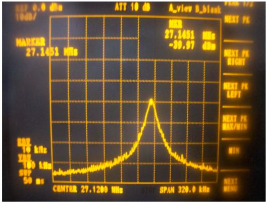
The results: The unit does meet the FCC Part 15 C requirements.
