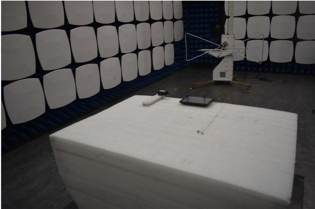
4. Radiated Field Strength Measurement(above 1GHz)
