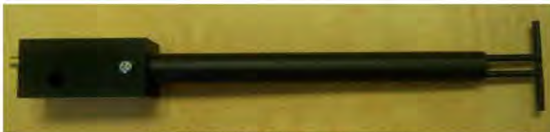
Figure 1 – MVG COMOSAR Validation Dipole
