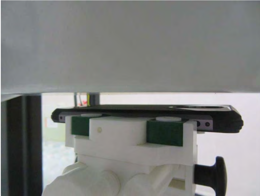
10mm body-worn Back Side Setup Photo (hotspot)
