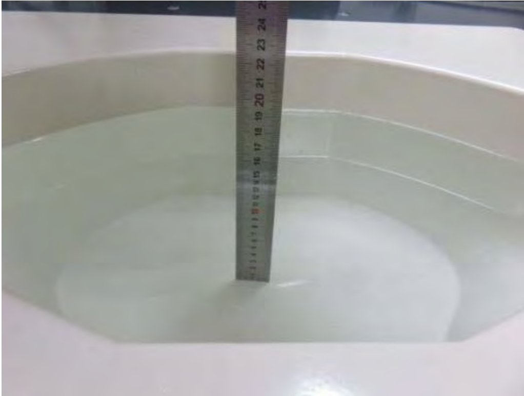
Photograph of the depth in the Body Phantom (835MHz, 15.2cm depth)
