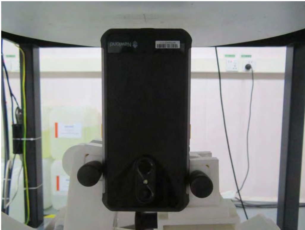
10mm body-worn Bottom Side Setup Photo (hotspot)
