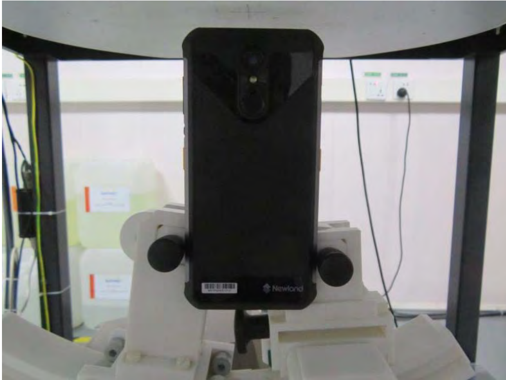
10mm body-worn Top Side Setup Photo (hotspot)
