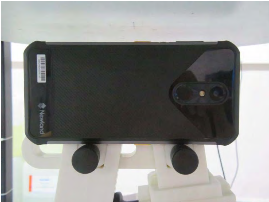
10mm body-worn Right Side Setup Photo (hotspot)
