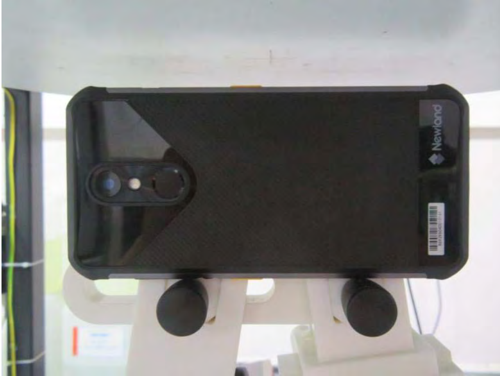
10mm body-worn Right Side Setup Photo (hotspot)
