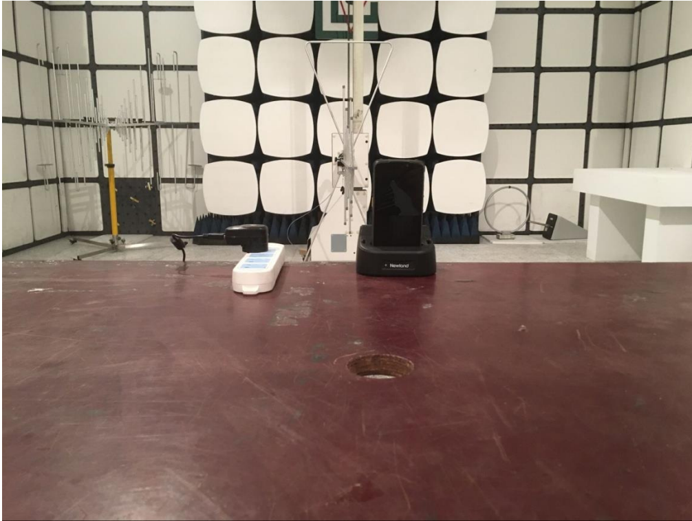
Radiated emission below 1GHz-charging from docking station
