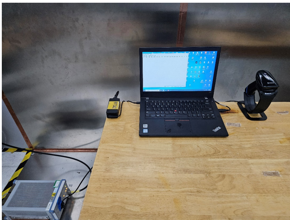
Photograph 3: Set-up for Conducted Emission on AC Mains
