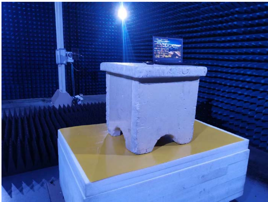
Photo of Radiated Emission Measurement Above 1GHz
