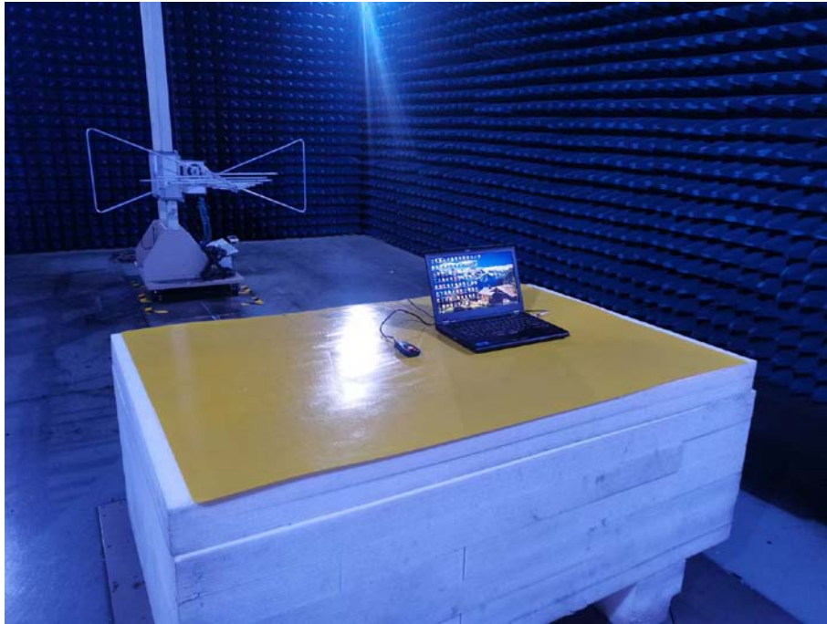
Photo of Radiated Emission Measurement Below 1GHz
