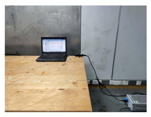
Photo of Power Line Conducted Emission Measurement
