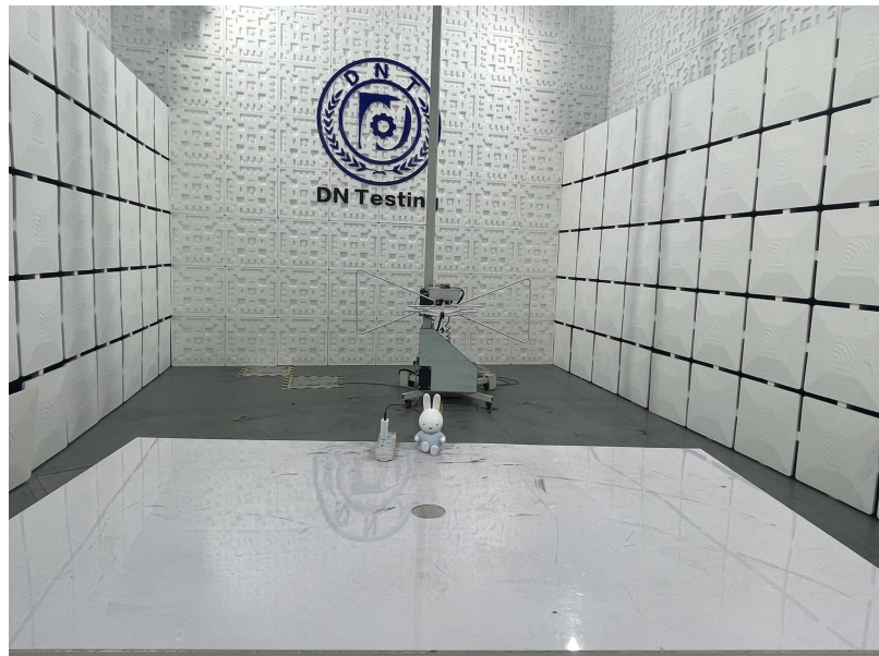
Radiated Emission Test View|(Below 1G)
