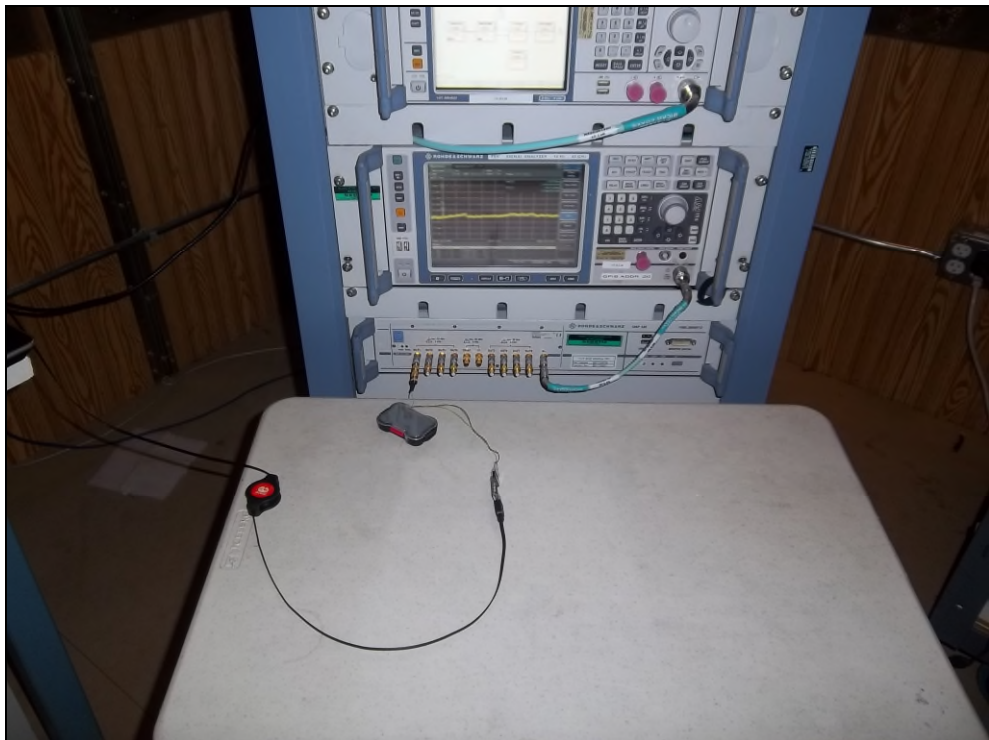
Figure 9: Equipment Under Test – RF Conducted Emissions
