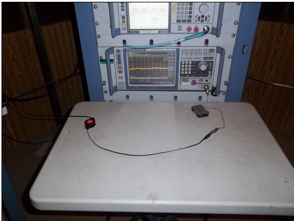
Figure 8: Equipment Under Test – RF Conducted Emissions
