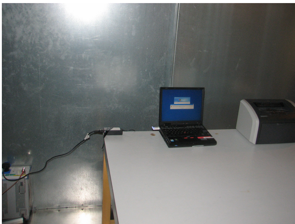
Set-up for AC Mains Conducted Emission
