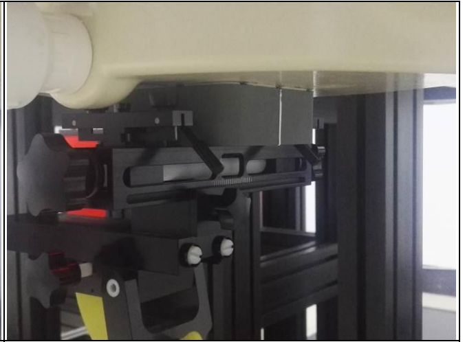
Rear Side of EUT with 0 cm Gap
