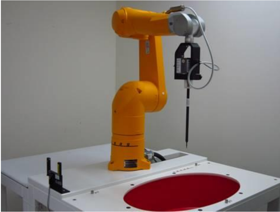
Fig.1 Photograph of the SAR measurement system
