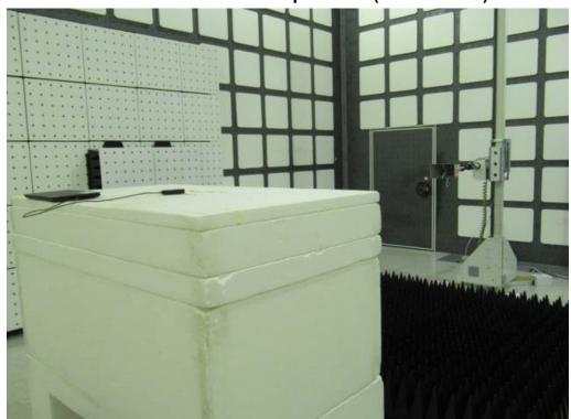
Radiated Emission Set up Photos (Front View)
