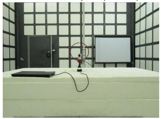
Radiated Emission Set up Photos (Below 1GHz)
