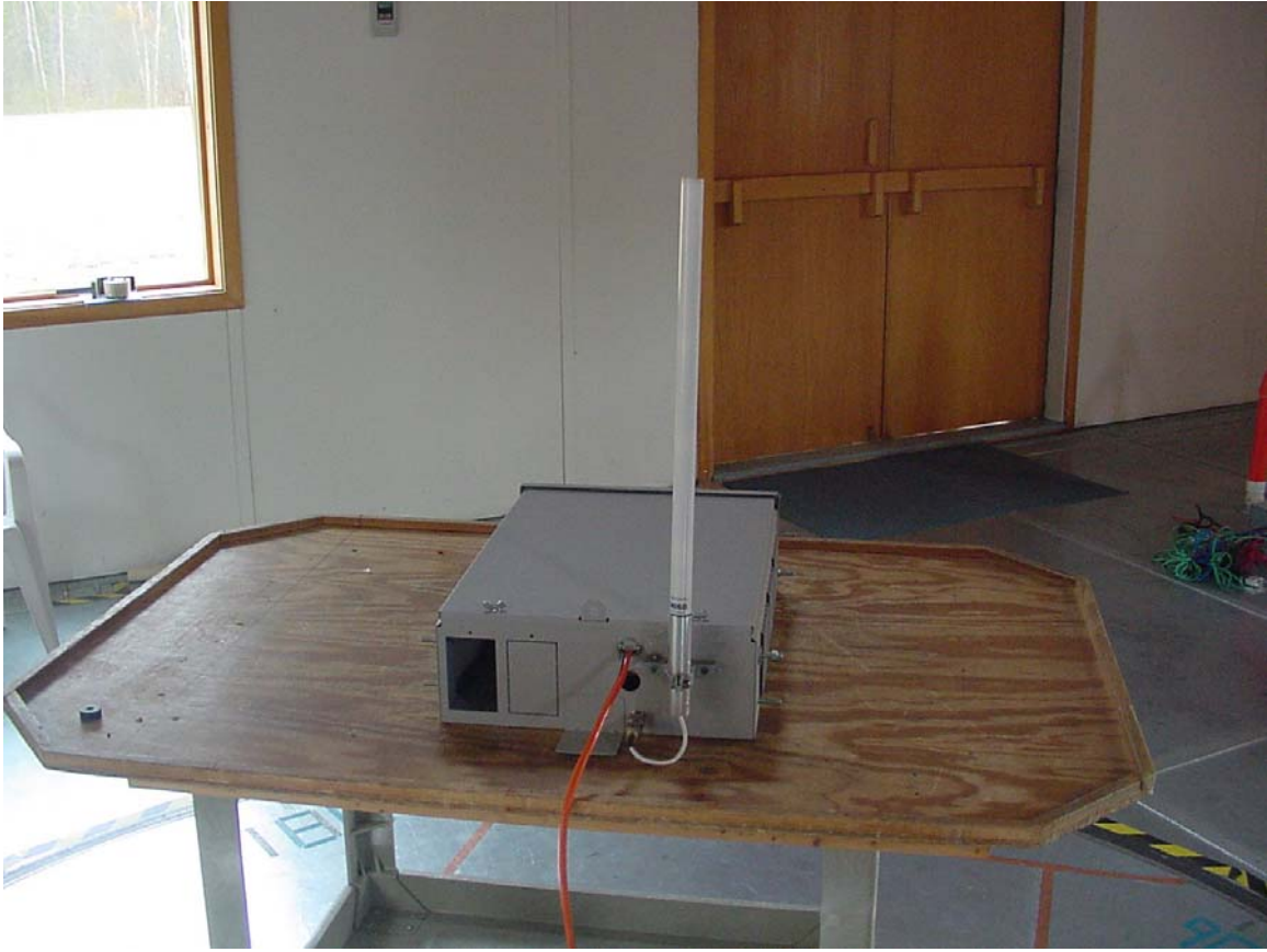
Radiated test setup rear with 6 dBd omni antenna
