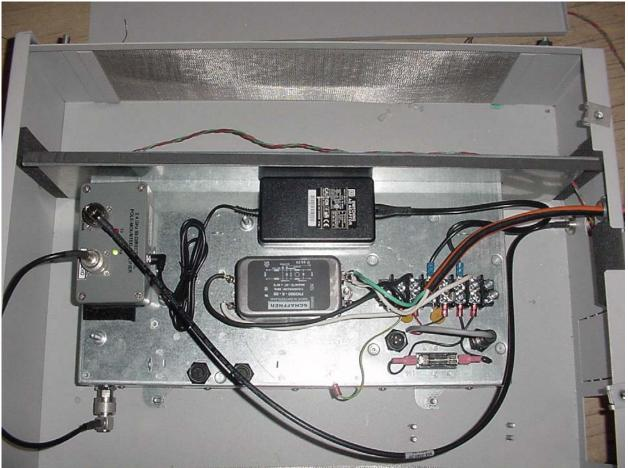
Photo shows the installation location of the schaffner filter inside the NEMA enclosure.
