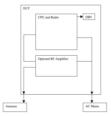
Note: If the RF amplifier is not included in the system, the cable that is used from the RF amplifier to the enclosure is connected directly to the radio and the radio to amplifier cable is simply deleted from the system.
